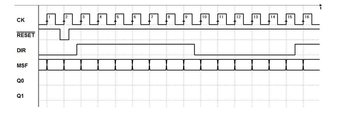
Chapter 7 – Exercise 1 – FSM Design Based on Textual Specifications – Timing Diagram to be completed
