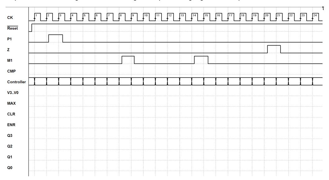
Chapter 8 – Exercise 5 – Design of the controller of a given datapath – Timing diagram to be completed
